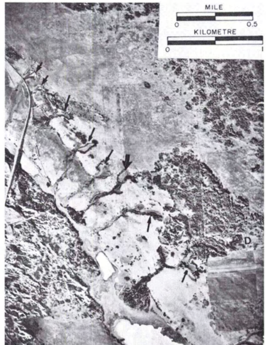
FIG. 8. Springs (arrows) formed by natural piping and erosion along the contact between a surface sand outwash (OW) and underlying till. Where the water table is high surface erosion is minimal. Where the water table is low the sand has been formed into dunes (D). Photo courtesy Canada National Air Photo Library.
