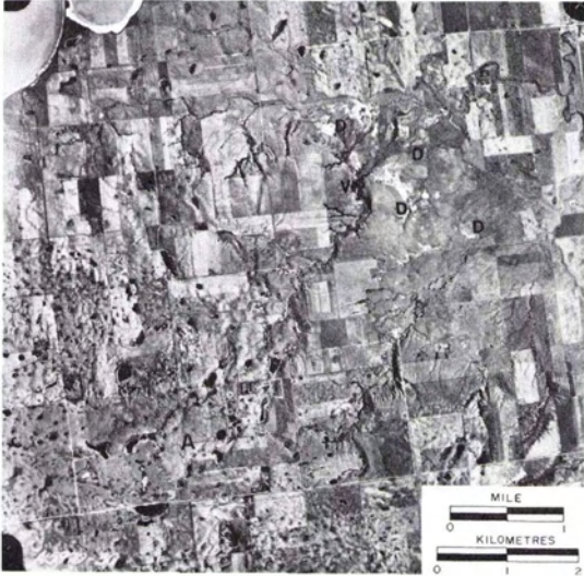
FIG. 12. A high relief ground moraine (A) is functioning as a ground-water recharge area. The area in the upper right half of the photograph is sloping away from the moraine and ground water is discharging at the base of the slope as indicated by saline patterns at D and the vegetation pattern at V.
