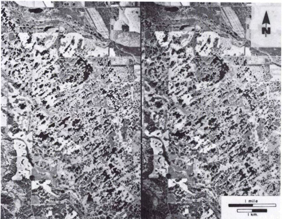
FIG. 3. A stereogram of a low relief (5 to 10 m) ridged moraine composed mainly of a thin (2 to 10 m) layer of clay rich till. Surface storage capacity is fairly large so recharge is significant even though the permeability of the till is low. The thin surface layer of till allows relatively efficient recharge of underlying sands or gravel. Photos courtesy Canada National Air Photo Library.
