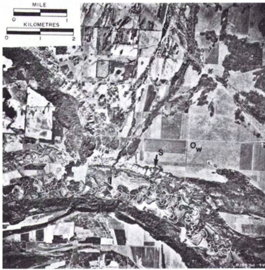
FIG. 5. A large outwash plain (OW) along the flank of a deeply incised meltwater channel. The sand and gravel layer is about 5 m thick and is an unconfined aquifer. Springs (S) can be seen on the valley slope where sand overlies till. Photo courtesy Canada National Air Photo Library.
