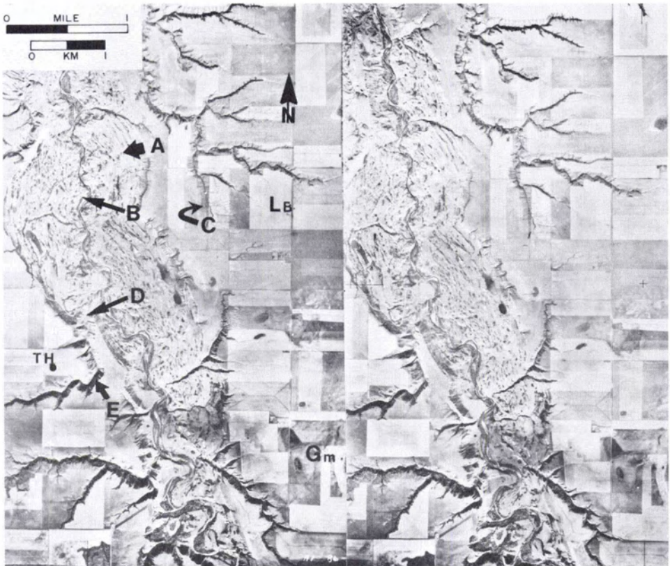
FIG. 16. Continuous retrogressive failure in soft clay shale can be seen in this stereogram at A and B. The elevation of the contact between the till and the shale can be seen at D. A lake basin clay at the surface is indicated by the gullies and tone patterns at C. The lake basin clay overlies till of a ground moraine exposed at Gm. Some seepage is evident at A. Photographs courtesy Canada National Air Photo Library.
