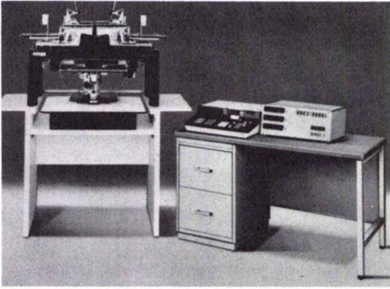
FIG. 4. Zeiss (Oberkochen) Planitope with DIREC-1 Display and HP-9810 Desk-Top Computer.
