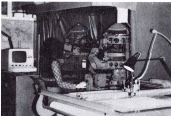
FIG. 7. Wild A8 with alphanumeric VDU for prompts and messages (Hunting Digital Mapping System).
