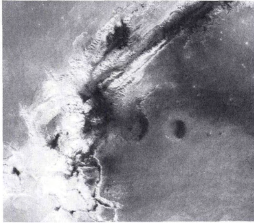
FIG. 6. Estimate of the average scene brightness R(x, y, \lambda_{red}) , which reflects only the intrinsic properties (albedo and color) of the materials within the scene. Coverage same as that of Figure 5.
