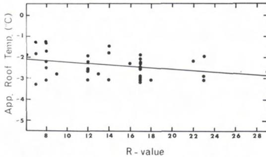
FIG. 3. Variation of apparent roof temperature with attic insulation levels for two-story houses.
