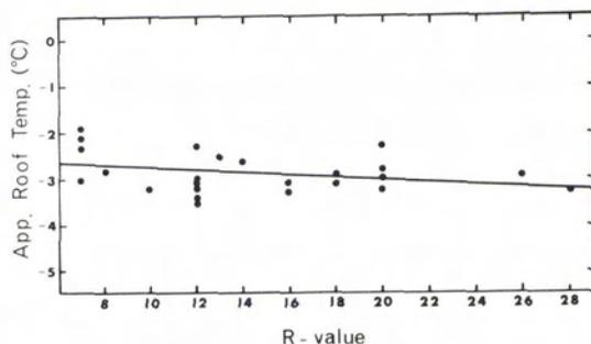
FIG. 2. Variation of apparent roof temperature with attic insulation level for bungalows.
