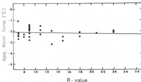
FIG. 4. Variation of apparent roof temperature with attic insulation levels for one-and-a-half story houses.
