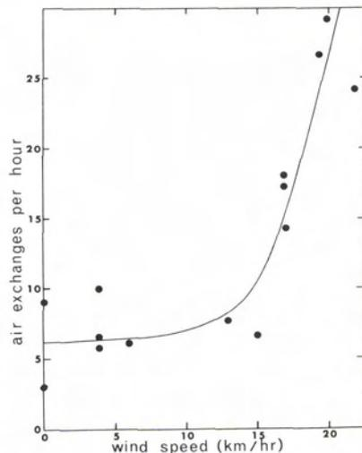
FIG. 5. Variation of attic air exchange rate with wind speed for test house.
