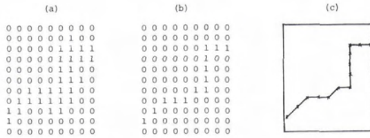
FIG. 2. Sketch explaining raster-to-vector conversion: (a) raster data structure, (b) skeletonizing as one example of the conversion, and (c) vector format.
