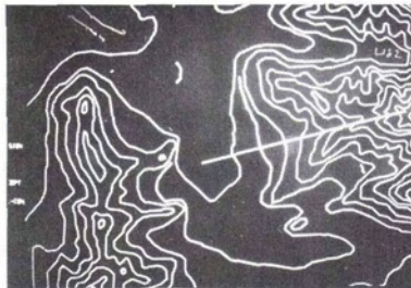
FIG. 11. Assigning heights to a number of contour lines in one step using a straight auxiliary line (locator). The lowest and highest contour get their height manually; intermediate contours are assigned automatically.
