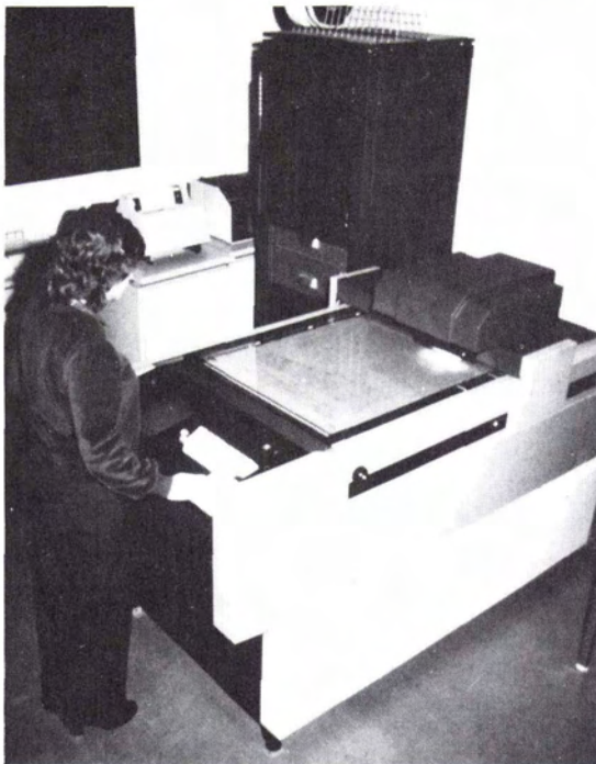
FIG. 7. KartoScan raster scanner in operation, recording output on magnetic tape.
