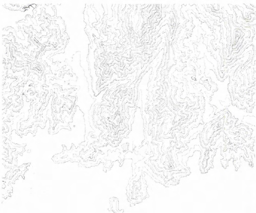
FIG. 18. Quality control of the height grid, using a rapid simple contour interpolation routine. The grid was generated using only contours.
