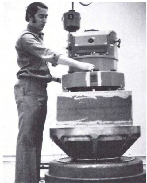
FIG. 5. Shaker arrangement for vertical vibration.
