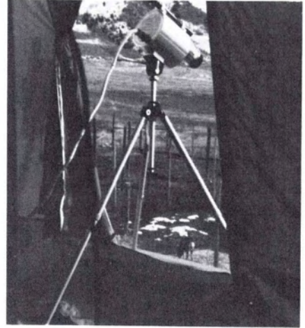
FIG. 4. The cvf spectrometer system mounted on the tower for the field experiment.
