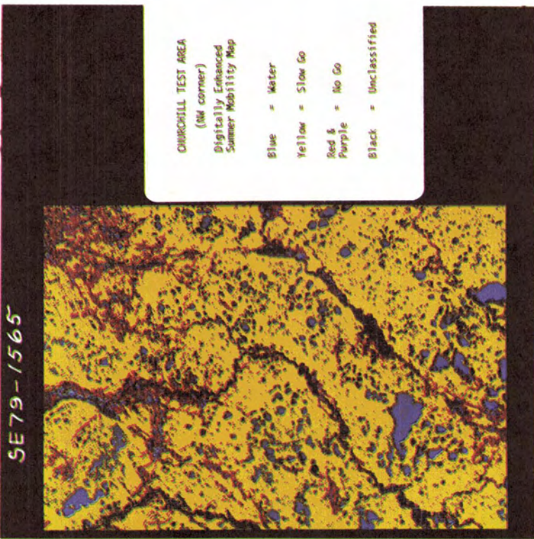
PLATE 1. Summer mobility map derived from unsupervised cluster analysis of selected Landsat mss bands. (Mobility interpretation: purple, red, and blue = "no go," yellow = "slow go," and black = "go.")
