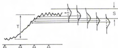
FIG. 6. The distribution of "field" pixels moves down the transition curve as the measurement point moves toward the boundary. The shaded area is the proportion which will be correctly classified.
