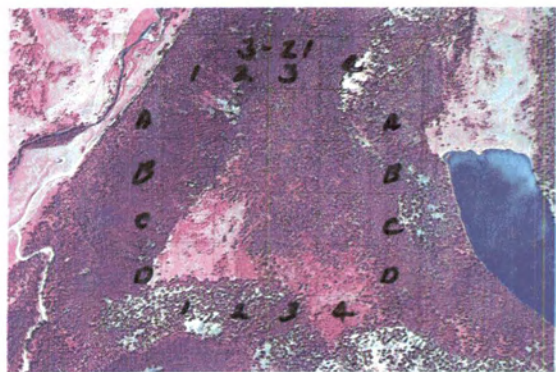
PLATE 3. Portion of infrared panoramic frame overlaid with 160-acre grid divided into sixteen 10-acre square plots.
