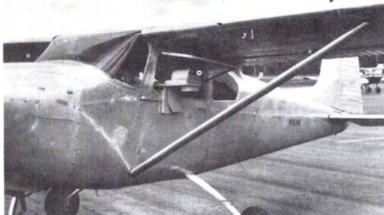
FIG. 2. Camera system and mount in position on a Cessna 182.
