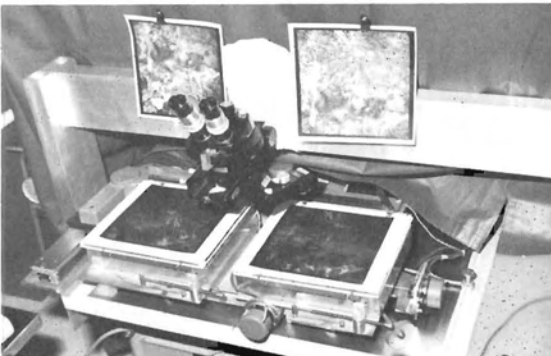
FIG. 2. Stereoscope, image holders, and encoders.
