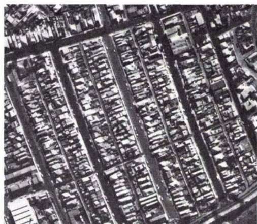
FIG. 4. High density residential ground truth area. Total area covered is 40 Landsat pixels, 8 along scan by 5 across scan. The scan direction of Landsat is from left to right.
