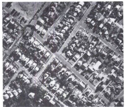
FIG. 3. Low density residential ground truth area. Total area covered is 40 Landsat pixels, 8 along scan by 5 across scan. The scan direction of Landsat is from left to right.
