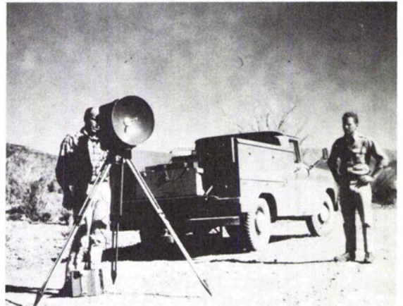
FIG. 6. USGS field party using EDM equipment.
