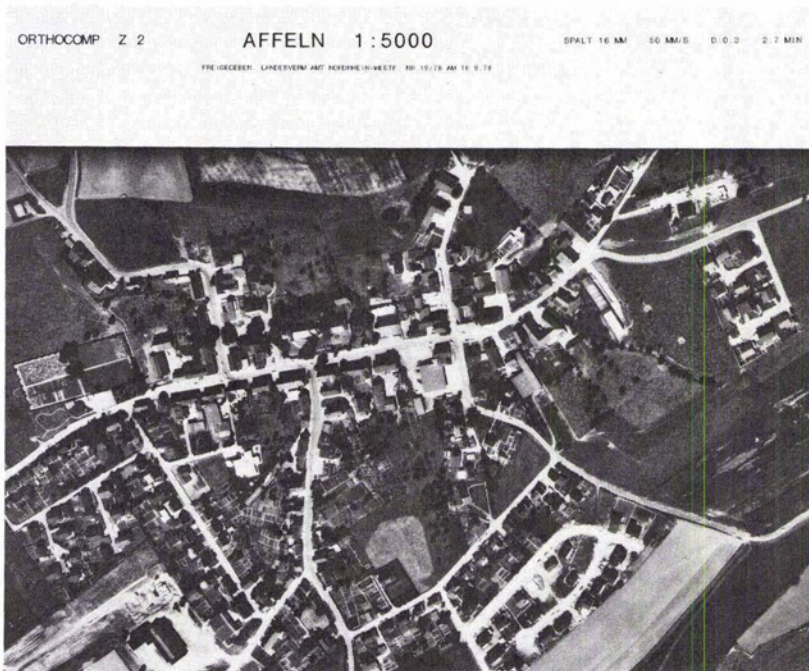
FIG. 3. Orthophoto with automatic print of marginal information generated with the Zeiss ORTHOCOMP (3:5 reproduction).
