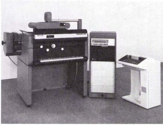
FIG. 3. Wild AVIOPLAN ORI with projection unit, process computer, magnetic tape station, and printer.
