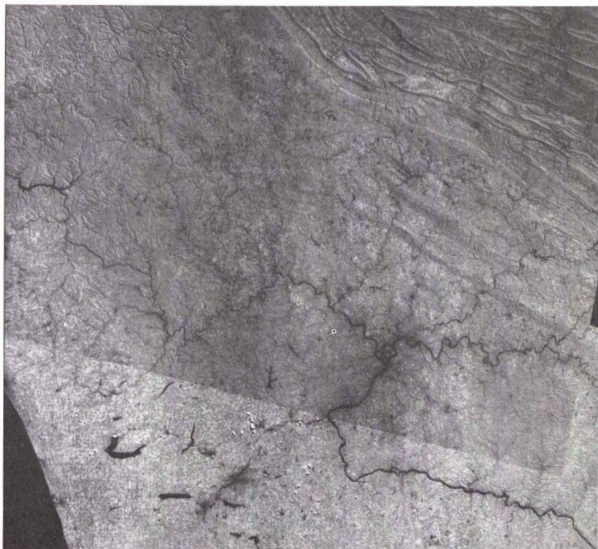
FIG. 5. The western portion of the State of Pennsylvania, UTM zone 17. Portions of six Landsat scenes of Band 6 (IR1) are shown here. The pixel resolution selected is 57 metres and is rotated so that north is vertical.
