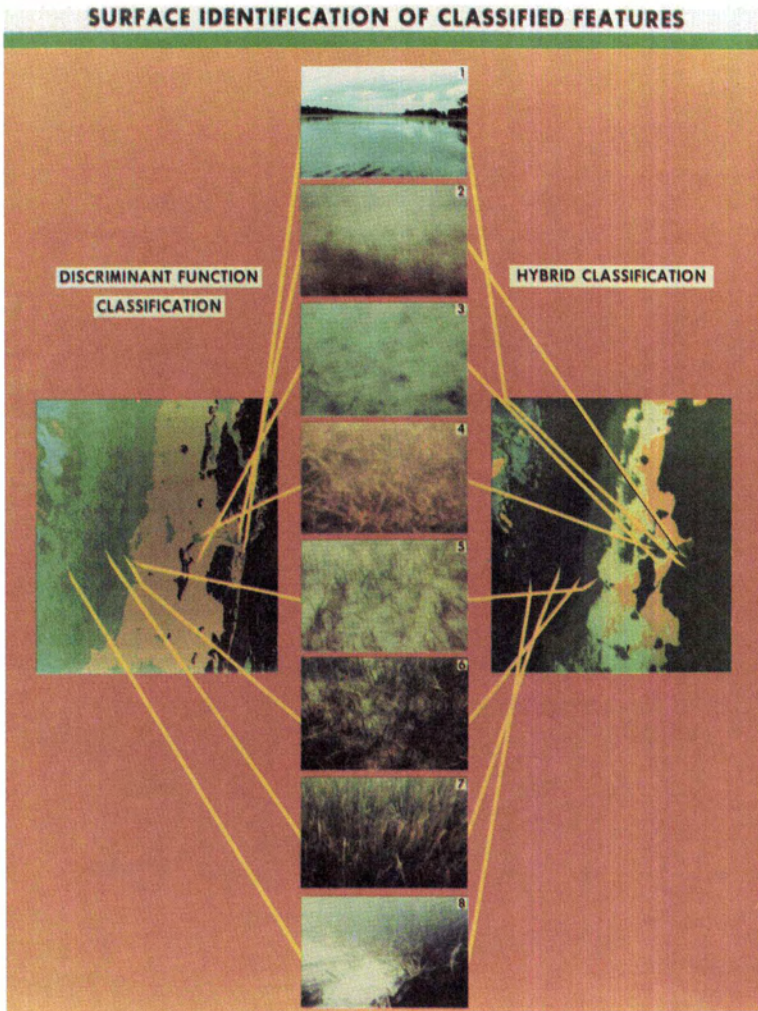
PLATE 5. Various bottom features of St. Joseph Bay, Florida, used in classifications together with their relative locations in submerged vegetation maps of the bay produced with the classification process.
