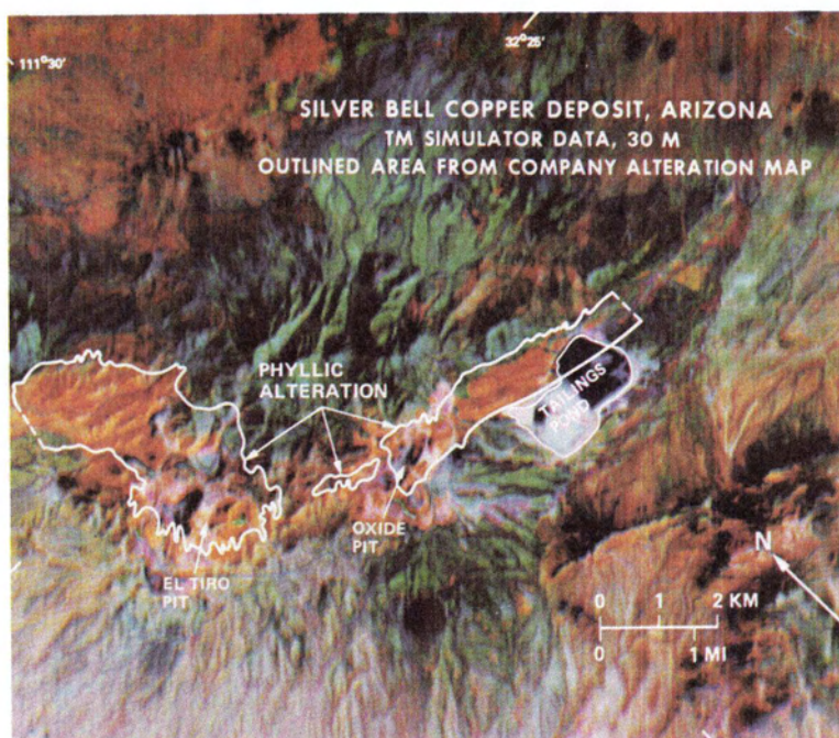
PLATE 1. Aircraft Thematic Mapper simulator data over the Silver Bell copper deposit, Arizona, resampled to 30-m pixels. Band ratios 1.6 \mu\text{m}/2.2 \mu\text{m} , 0.66 \mu\text{m}/0.56 \mu\text{m} , and 0.83 \mu\text{m}/1.65 \mu\text{m} displayed as red, green, and blue, respectively. The main alteration zone is displayed in yellow due to the presence of hydroxyl-bearing and iron oxide minerals. Data acquired 22 October 1978.
