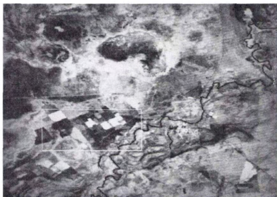
FIG. 1. (a) Band 7 Landsat MSS image of the region of the investigation, showing irrigated fields (white). The area enclosed by the white border is shown expanded in (b) and was used in signature generation.
