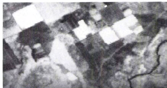
FIG. 1. (a) Band 7 Landsat MSS image of the region of the investigation, showing irrigated fields (white). The area enclosed by the white border is shown expanded in (b) and was used in signature generation.
