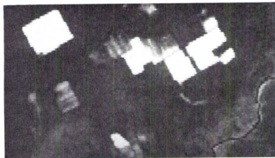
FIG. 8. Band 7/band 5 ratio of the region of Figure 1b generated with the real time look-up table manipulation facilities of the DIPIX image analysis system.
