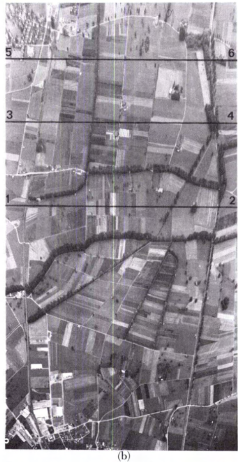
FIG. 7. (a) Extremely tilted aerial photograph taken with RC10 near Heerbrugg, Switzerland. (b) The same photograph after its rectification with the ORI/SORA-PR system (original scale 1:10 000). The basic magnification in the four areas formed by the lines 12, 34, and 56 has been changed manually during scanning.
