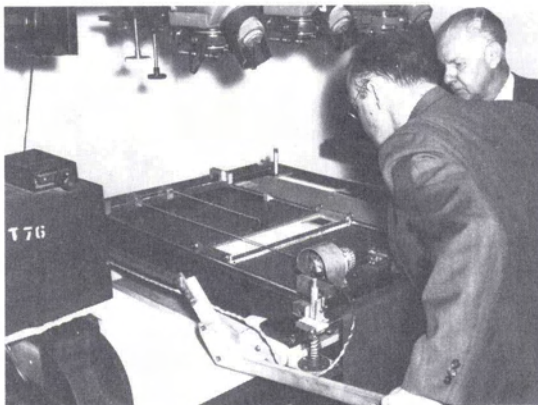
FIG. 12. This breadboard model orthophotoscope being tested by R. B. Southard, Jr. who later became Chief, National Mapping Division, and R. K. Bean. It was developed by R. K. Bean and his research team in the mid-1950's. This USGS orthophotoscope and later models were the first to economically produce orthophotographs that met the horizontal accuracy requirements of the National Map Accuracy Standards.
