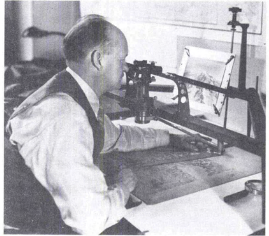
FIG. 3. Plotting Alaska map detail with a Wilson photoalidade, designed by R. M. Wilson in 1932. Its precursor was a panoramic photoalidade developed by J. W. Bagley between 1910 and 1916. The illustrated instrument is operated by Gerald FitzGerald who later became Chief Topographic Engineer of USGS and 12th President of the American Society of Photogrammetry. This same instrument No. T.1. was the one whose facility for measuring on oblique photographs sparked the idea which grew into the Trimetrop System.
