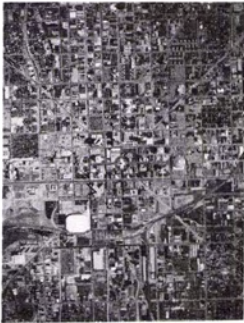
FRONTSPICE PHOTO—Indianapolis, Indiana, taken July 1984 using a Zeiss RMKA camera with a 152mm lens and 2445 color film.
