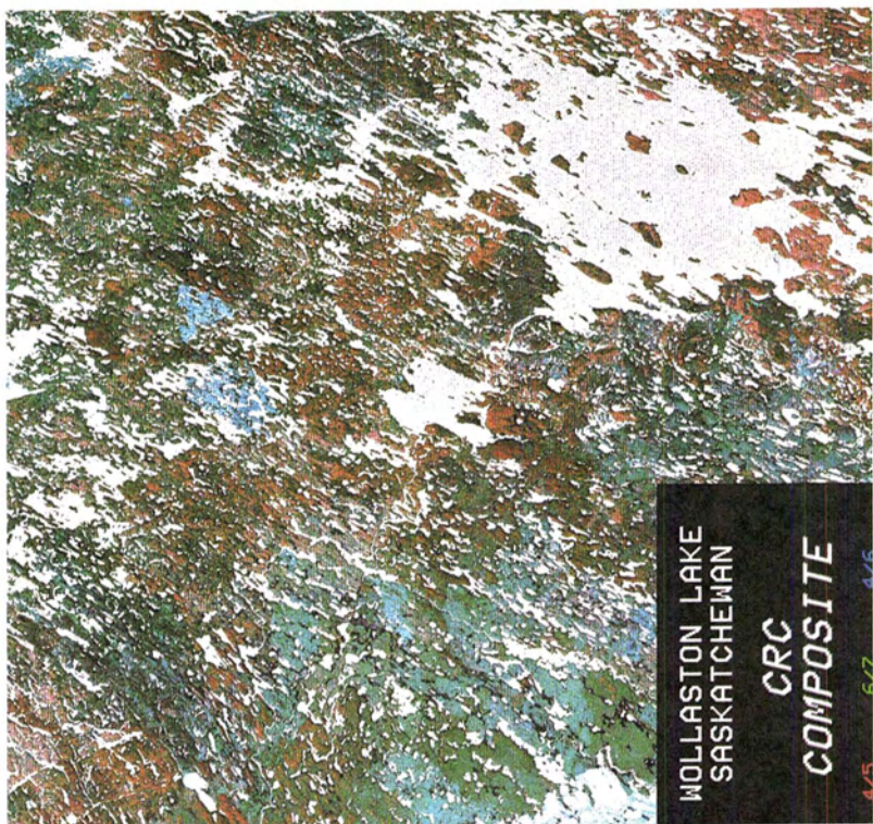
PLATE 2. Landsat color-ratio composite image of the Wollaston Lake area, Saskatchewan, Canada. A 2 percent linear stretch about the median ratio DN, based on the rock/soil histograms, was applied to each of the band ratios. Distance across the top of the title block is 56 kilometers.
