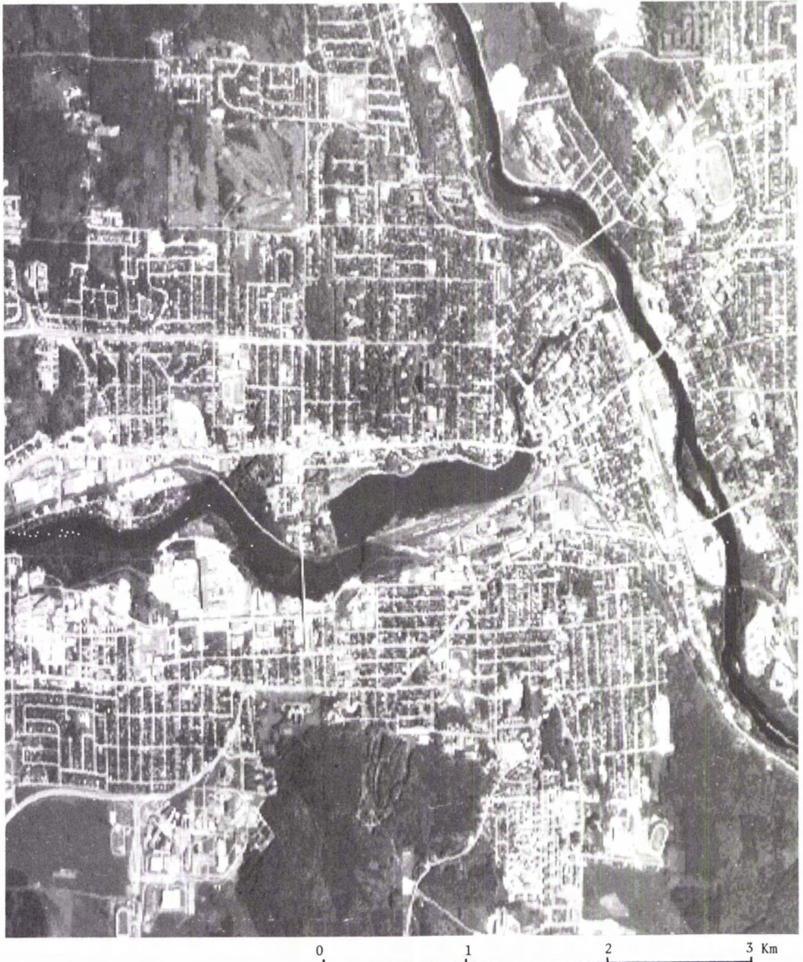
FIG. 1. Simulation of SPOT panchromatic channel imagery with 10-m resolution over the city of Sherbrooke, Quebec.
