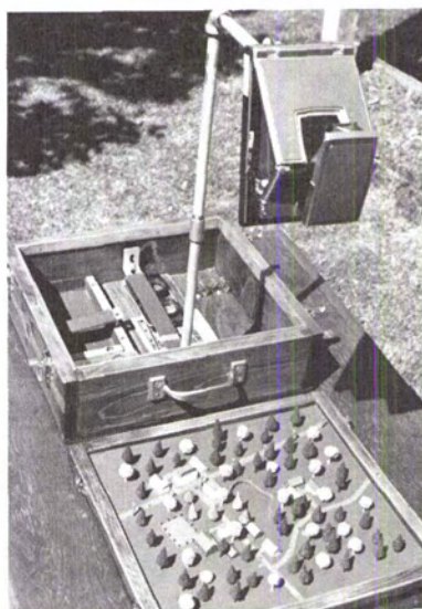
FIG. 3. The stereo kit prepared for operation. The terrestrial model is actually the underside of the cover. Note the circular bubble level on the lower left side of the camera.
