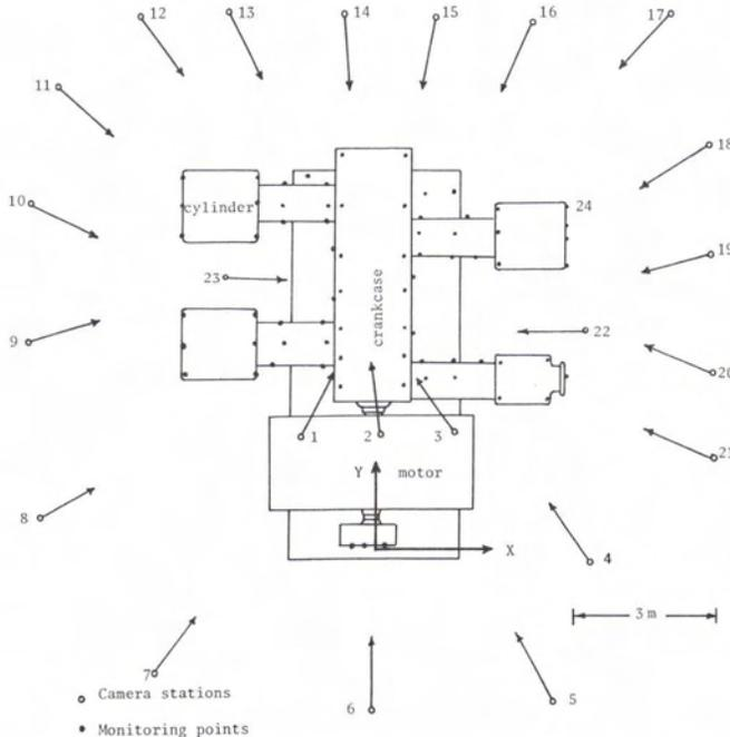
FIG. 2. The geometric configuration of the 23 camera stations.
