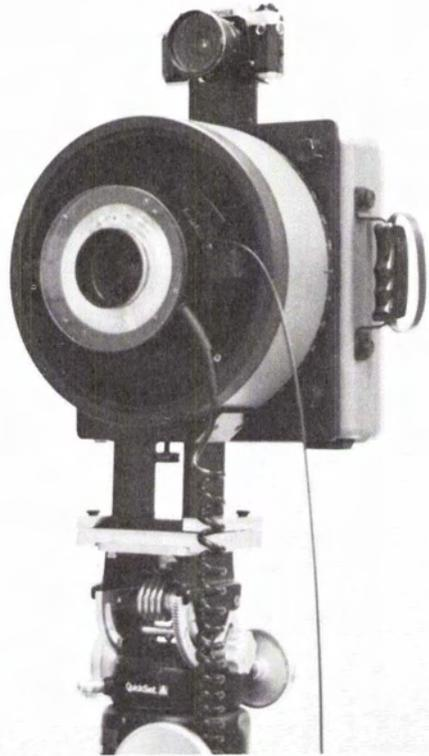
FIG. 4. The CRC-1 camera with 120-mm lens and ring strobe.
