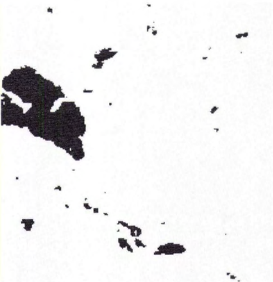
FIG. 2. The class "water" is separated from the other classes and shown as a binary image, with water in black and the rest of the mapped image in white. Each class is mapped in this manner.
