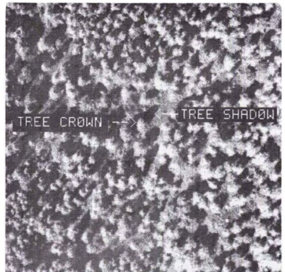
FIG. 2. Example of electrostatic plotter output for Channel 9 of the MSS data.
