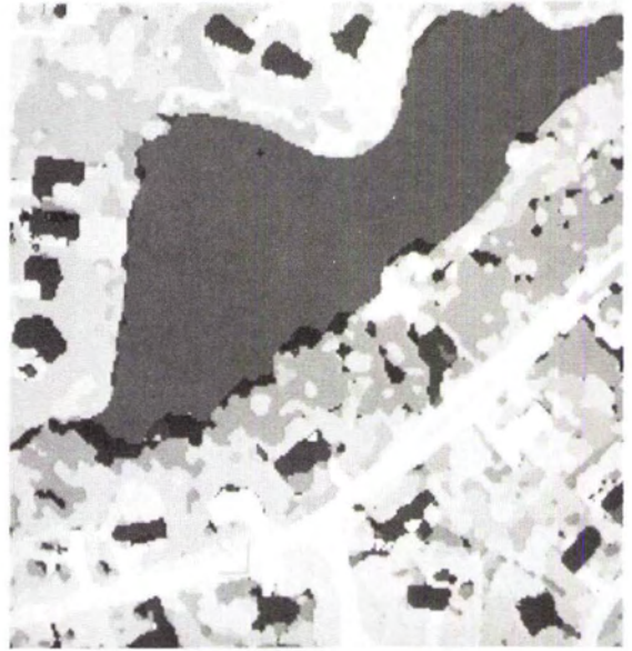
FIG. 8. Computer classification after three iterations with the majority rule smoothing operator — parallel processing.
