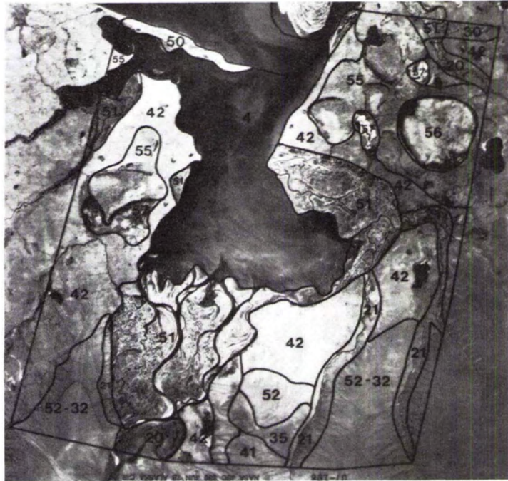
FIG . 6. Preliminary photo-interpretive mapping product to be verified. Map unit labels correspond to the range sites listed in Table 1.
