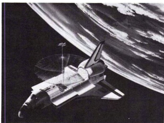
FIG. 9. Artist's rendition of a large hoop-column antenna deployed on the space shuttle (photo courtesy of NASA-Langley Research Center).
