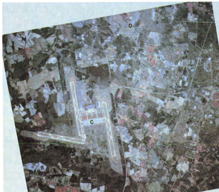
FIG 4. Landsat TM bands 2, 3, and 4 plus the NHAP photograph false color composite. This is the same product as Figure 3 but with the NHAP photograph added, pixel-by-pixel, to the TM data before compositing. The scale of the image is 1:80,000. See Figure 1 for feature identification. (Reduced to a scale of 1:135,000 for publication.)
