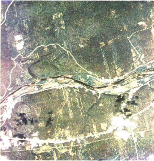
PLATE 1. Contrast-stretched natural color composite image formed from MEIS-II band 2 (0.51 to 0.54 micrometres) displayed as blue, band 3 (0.58 to 0.61 micrometres) displayed as green, and band 4 (0.66 to 0.69 micrometres) displayed as red. Resolution 7 m.
