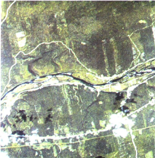
PLATE 3. Color composite image formed from Daedalus MSS band 4 (500 to 550 nm) displayed as blue, band 5 (550 to 600 nm) displayed as green, and band 7 (630 to 700 nm) displayed as red. These data have been radiometrically matched to the data displayed in Plate 1 as described in the text.
