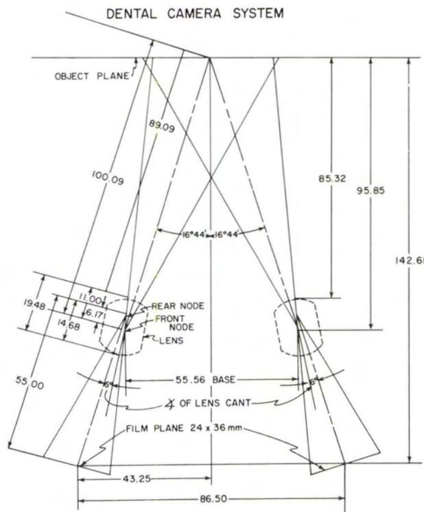
FIG. 1. Camera interior and exterior geometry.
