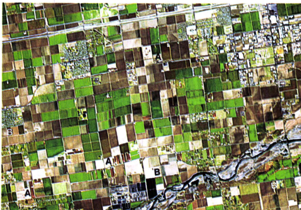
PLATE 1b. Color composite of TM bands 1, 4, and 5 merged with the SPOT panchromatic band for the agricultural site. The vegetation is green because TM band 4 was used as the green component. The print is labeled for comparison with Plate 1a. The three A's are showing some of the red hues in the fields. The three B's are showing some of the hues that are different or unique compared to their hues in Plate 1a. Copyright SPOT data CNES; TM data reproduced with permission of EOSAT.
