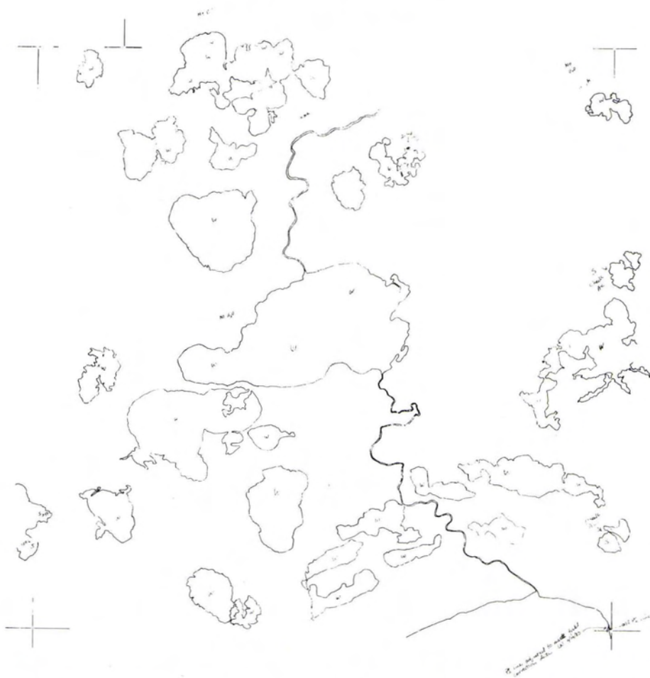
FIG. 2. Photo interpreted manuscript for T. 1 S., R. 82 W., Seward Meridian, Alaska. Based on Figure 1 and color infrared photography and used to produce data for the ARSUP database.
