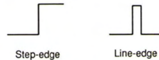
FIG. 3. Examples of edge-profiles before 'blurring' by the Imaging System (after Nalwa and Binord, 1986).
