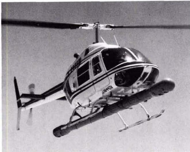
FIG. 1. The stereo-boom mounts longitudinally on a small helicopter. Metric, 70-mm Hasselblad cameras are mounted in each end (note holes). Cameras are operated from the cockpit.
