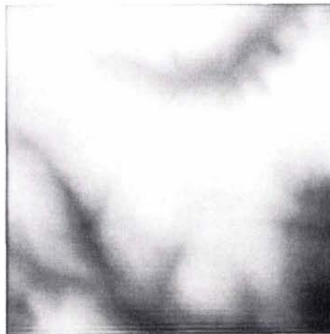
FIG. 12. Radar shape-from-shading height model with the height linearly mapped into brightness values for comparison with the photogrammetric data set in Figure 10. Again, note the improved similarity with the photogrammetric data, when compared to the less accurate data of Figure 1 from radar stereo.
