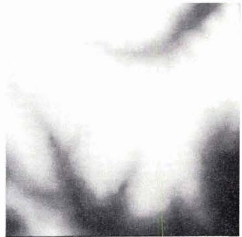
FIG. 10. Photogrammetric height model with the heights linearly mapped into brightness values. Source: Aerial wide-angle photography at a scale of 1:50,000, permitting an accuracy in height of the Digital Elevation Model of about \pm 1 m. Area is 3km by 3km, covering a segment of Brazeau for comparison with the radar images in Figures 4 and 5.
