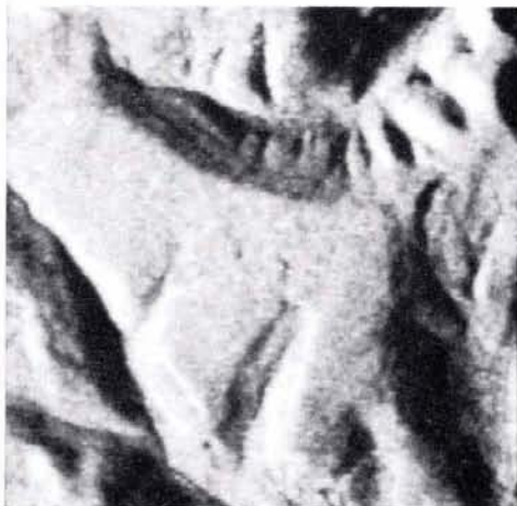
FIG. 4. Ortho-rectified input radar image (Area: East of Brazeau Range, Canada. Pixel size = 24 m; Size of area - 128 by 128 pixels or 3km by 3km). Radar image produced by Intera Technologies Ltd., Calgary, Canada, using the STAR-2, X-band SAR with 6-m resolution at seven looks. Look angle off-nadir approx. 71°.
