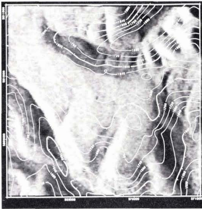
FIG. 8. Radar stereo derived contour lines are superimposed over the rectified radar image in Figure 4. Contour line interval is 40m; contours are computed from the Digital Elevation Model. Note the fact that the contour lines fail to model geomorphological structure, e.g., in the upper right corner of the 3km by 3km area.
