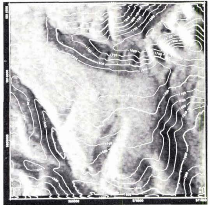
FIG. 9. Radar shape-from-shading derived contour lines are here superimposed over the radar image of Figure 4. Comparison with Figure 8 reveals an improved modeling of geomorphological structure. Contour interval is also 40m. Ringing effects along the edge of the area are artifacts.
