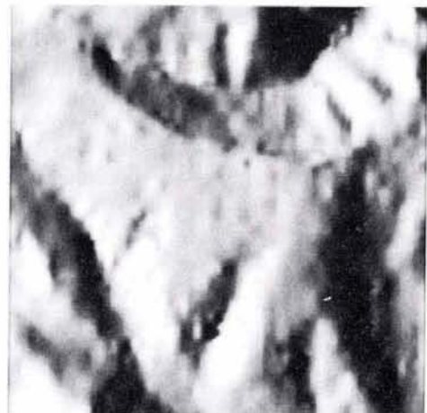
FIG. 6. Illuminated radar stereo derived height model using the images in Figures 4 and 5 as input, together with Global Positioning System navigation data. Illumination angle is 58° to obtain similarity to SAR images. Terrain height differences are about 478 m. RMS height errors were determined by comparison to a map and amount to \pm 25 m. Note that this error causes a neglect of morphological detail. Spacing of the stereo measurements was about 250m.
