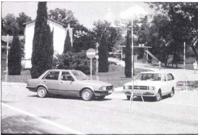
Fig. 4. A photograph of a simulated accident site taken with a non-metric 35- to 70-mm zoom camera, showing "preferred" range pole arrangement.
