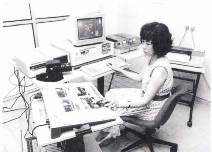
Fig. 5. Enlarged positives arranged on the digitizer for on-line data ( x, y ) acquisition.
