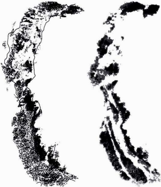
FIG. 6. Comparison of La Jolla kelp distributions during fall 1987 derived from CIR aerial photographs and SPOT HRV-XS digital data. Figure 6a was manually traced from CIR aerial photographs taken on 10 September 1987 (W. North, unpublished map, 1987). Figure 6b was derived from an XS3/XS2 band ratio of the SPOT digital data acquired on 10 October 1987. Absence of canopy in the central area of Figure 6b is primarily due to kelp harvesting between dates.
