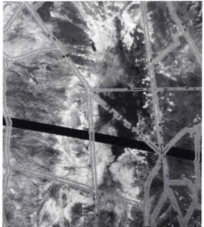
FIG. 2. Classification map (75 classes) of Puddle Valley study area showing the results of the unsupervised classification of transformed TM imagery. The light gray strips represent the 270-m and 150-m buffer zones for known locations of nondieback. The dark gray areas within the light gray buffer zone represents locations of known shrub dieback. The pixel class frequencies within the buffer zone were used to determine which of the 75 spectral classes were associated with dieback. The wide diagonal black strip crossing the map is where 18 bad lines of the image were deleted from the original TM data.
