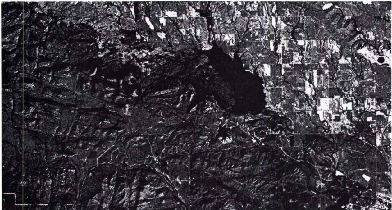
FIG. 2. Rotated Landsat TM band 3 image over a portion of the Wichita Mountains in southern Oklahoma. This image is 952 by 508 pixels at a scale of 1:160,380.
