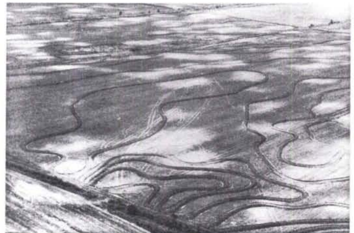
FIG. 3. Low aerial view of present day "sand blows" (light patches) in a rice field in southeastern Missouri. Most of the sand blows are about 5 m across. The contours are rice levees.
