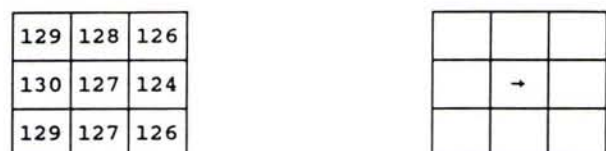
FIG. 1. A hypothetical example illustrating the raster principles of slope-line detection. The left shows the elevation data of a 3 by 3 kernel. An arrow indicating the direction of steepest descent is assigned to the central cell as shown on the right.
