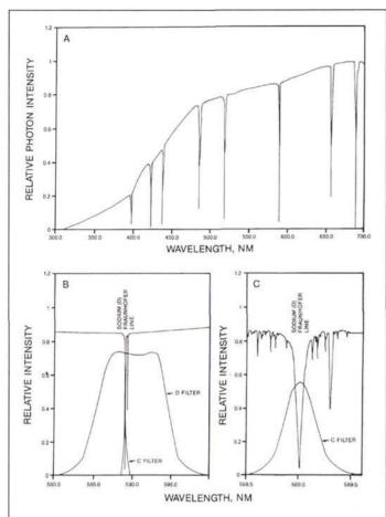
Figure 3. (a) Solar spectrum showing Fraunhofer lines, (b) relation between the sodium (D) Fraunhofer line and the D and C channel filters, (c) detail solar spectrum showing the Sodium (D) Fraunhofer line, C channel filter, and numerous absorption bands due to water vapor. Spectral data were obtained from the Kit Peak Observatory.
