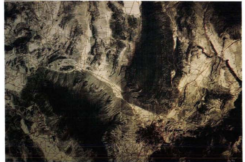
Plate 6. Hardcopy stereo image of the Las Vegas area in which TM band 3 and DLG data are combined. The original stereo data were generated by using the DEM to offset the TM and DLG, resulting in four images: left and right TM, and left and right DLG. These four images were combined as a single anaglyph image on an electrostatic plotter.
