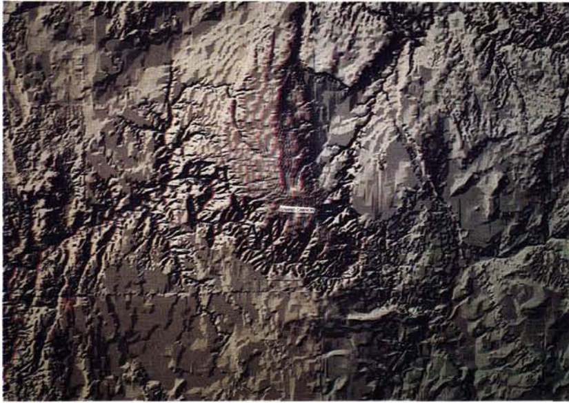
Plate 3. Hardcopy stereo image of part of the Grand Canyon area. The original image was electrostatically printed in anaglyph format at a scale of 1:250,000 in four panels and measures 3 m by 1.5 m.
