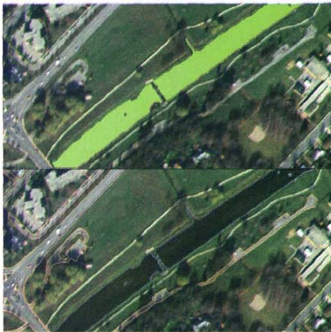
The process for automated extraction of spatial and spectral features is illustrated for the water area in this image. Boundaries of homogeneous features form the GIS polygons.
