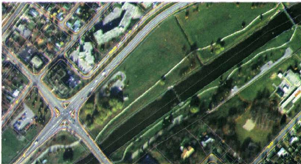
GIS features, such as streets, building, and parks are extracted from the MEIS data using computer-applied expert reasoning techniques. The process enhances efficiency in updating or constructing the urban digital map.
