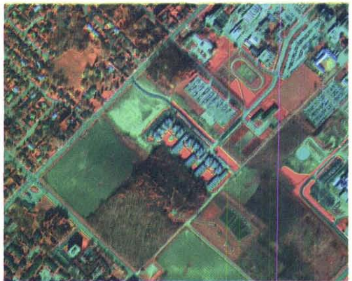
Three of the six MEIS calibrated spectral bands are employed to produce this false color digital image. The reflected infrared band enhances the red-encoded vegetation for computer-assisted feature extraction.
