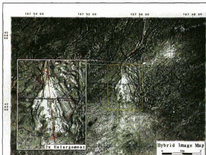
Plate 1. False-color-infrared "hybrid" image map of the Stratton Draw site. Its 10-m resolution is governed by the digitized aerial photograph (intensity). Color information (hue and saturation) is comparable to a Landsat MSS 7-5-4 (R-G-B) display. Shown are rough dissected terrain above the maximum level of the lake (A); remnant shoreline (B); spectrally homogeneous paleolake bed (C); and lake-marginal sand dunes (D) downwind of the delta. Heavier growths of sagebrush and grasses are revealed by red mottling. The triangular morphology of the delta and location of slope measurement sites (A to B) are shown on the 2x-enlarged (5-m pixel size) inset map.
